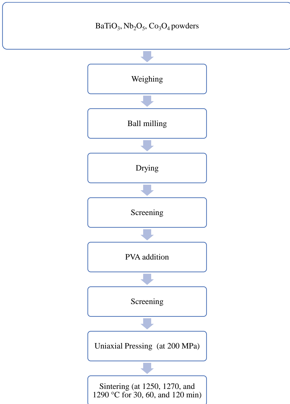
Figure 19. Flowsheet showing the steps applied for the preparation of the BaTiO 3 based ceramic capacitors.
